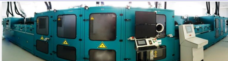
R2R Pilot Line equipped with Precision Metrology & Patterning Tools
